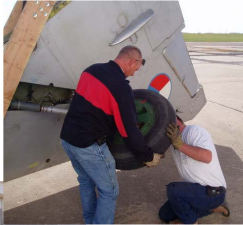
Above: Marty Batura and Bill Lemieux fit a wheel to a landing gear strut. Left: Less than 48 hours later, a freshly washed MiG-21 sits in front of 604.
